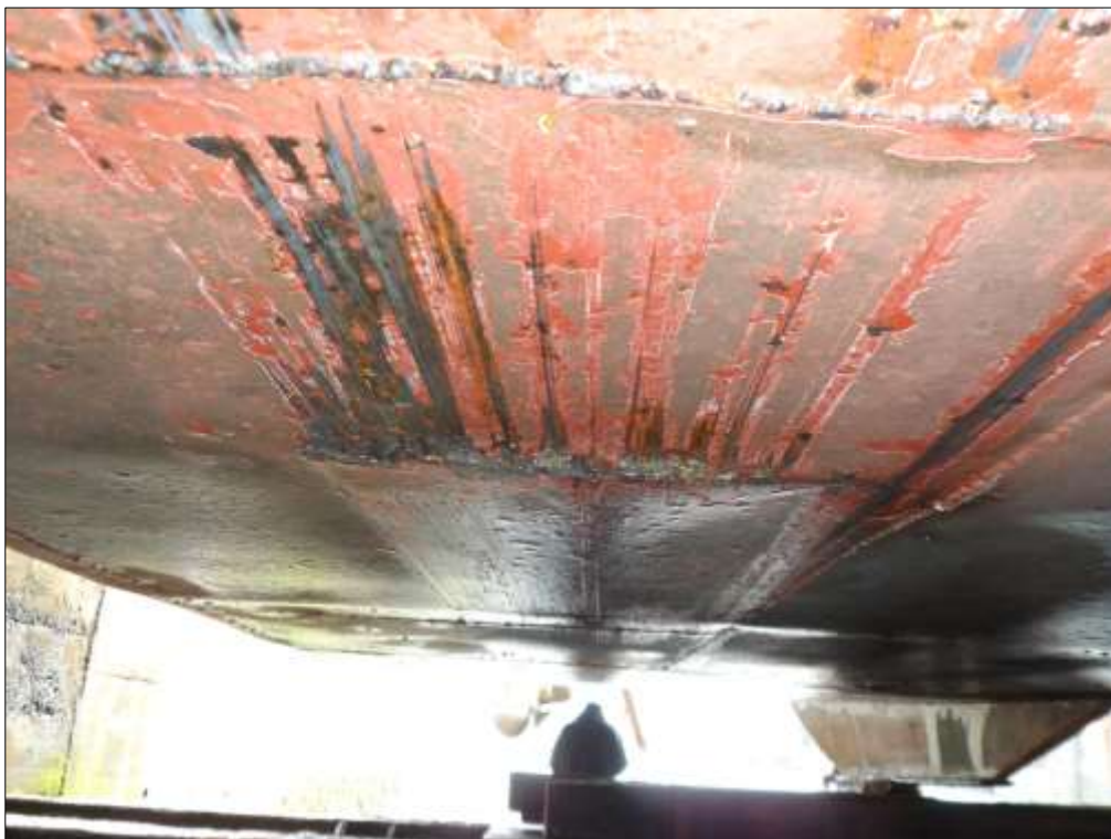
Figure 1: Shell plating damage to starboard hull
