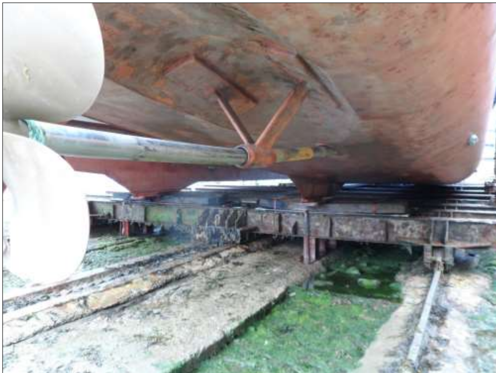
Figure 6: Starboard shaft and 'P' bracket distorted
