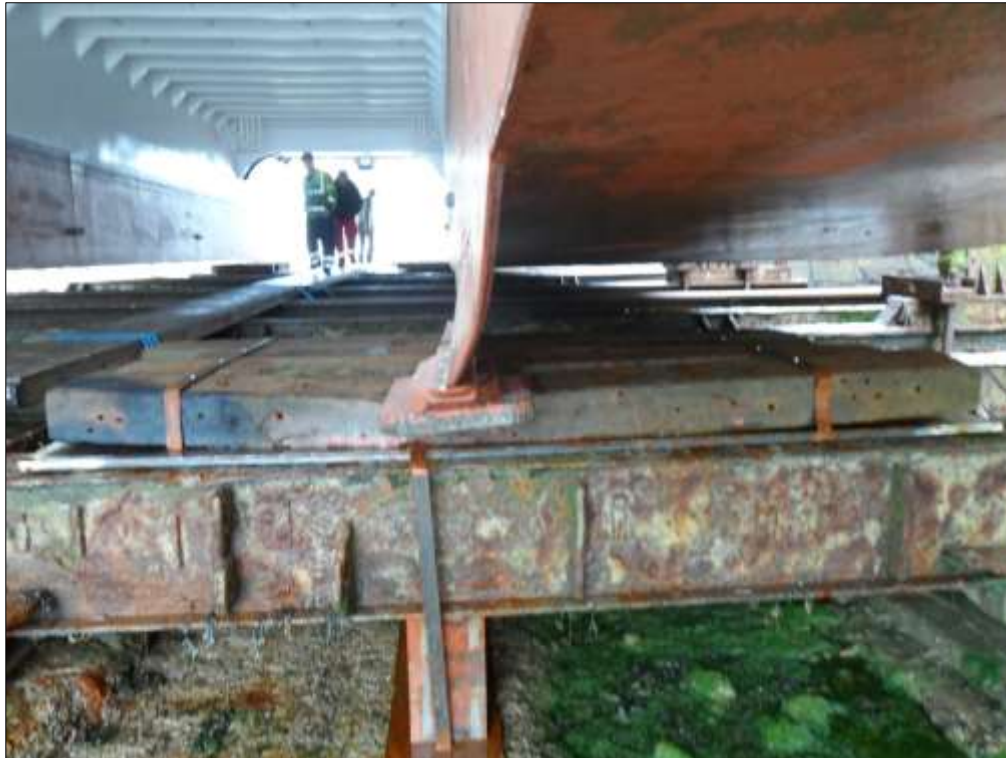
Figure 3: Distortion to starboard skeg
