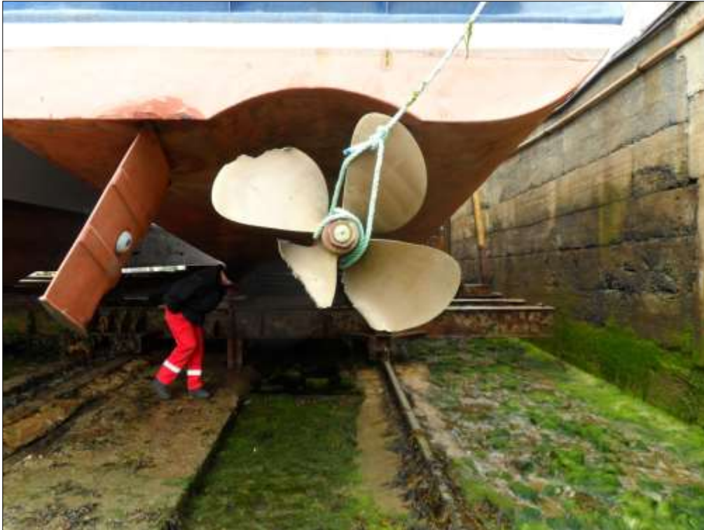
Figure 5: Starboard propeller blades heavily damaged or missing
