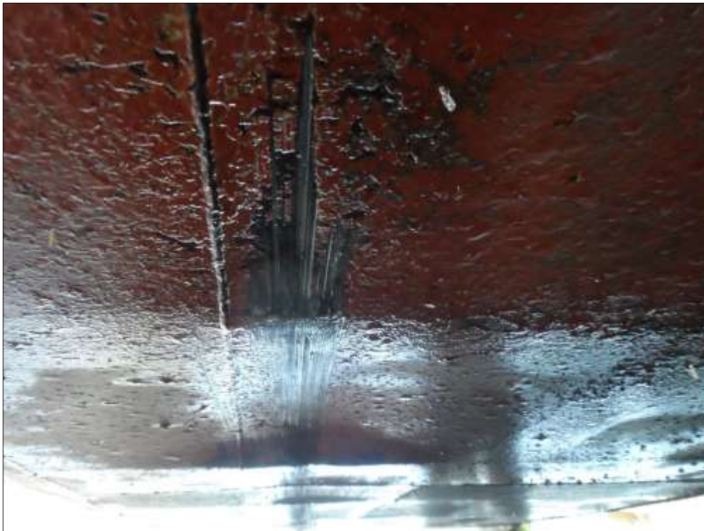
Figure 1: Shell plating damage to starboard hull
