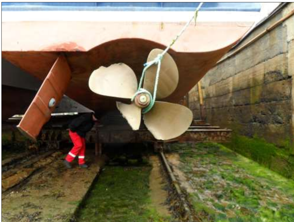
Figure 4: Starboard rudder distorted out of position
